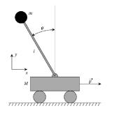
Goal: stabilizing around the goal  $(x = x^*, u = u^*)$  $c(x_h, u_h) = d(u, u^*) + d(x_h, x^*)$ minimize  $\mathbb{E}_{\pi} \Big[ \sum_{h=0}^{H-1} c(x_h, u_h) \Big]$ such that  $x_{h+1} = f(x_h, u_h), u_h = \pi(x_h), x_0 \sim \mu_0$
