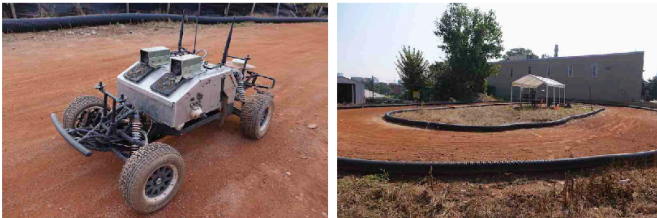
Fig. 4: The AutoRally car and the test track.
